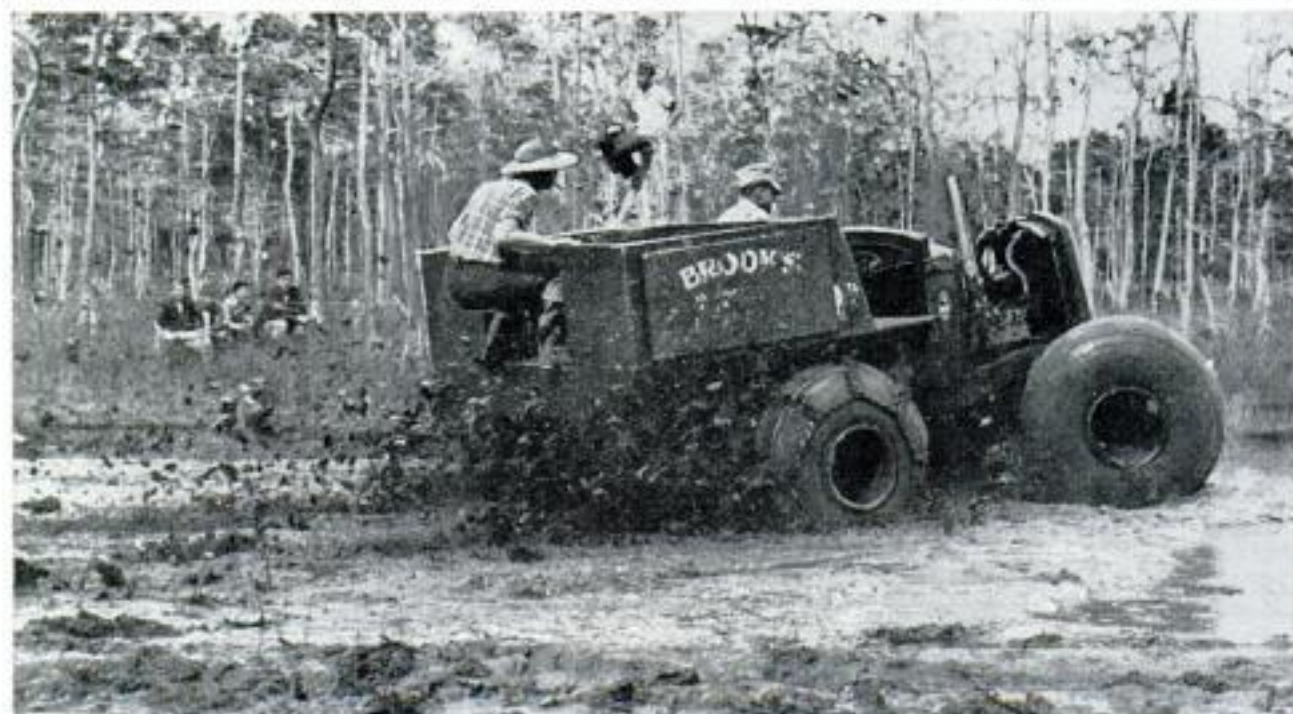
Man on rear of swamp buggy aids traction by shifting his weight around. Spinning tires send mud flying
